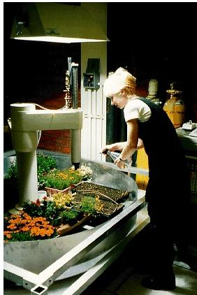
"The Telegarden is an art installation that allows web users to view and interact with a remote garden filled with living plants. Members can plant, water, and monitor the progress of seedlings via the tender movements of an industrial robot arm."
